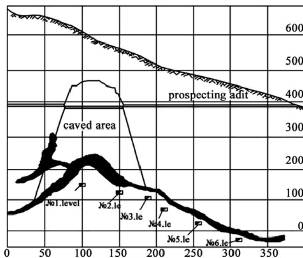
Figure 7. Sectional view of the mining panel caved in the 3<sup>rd</sup> gallery
