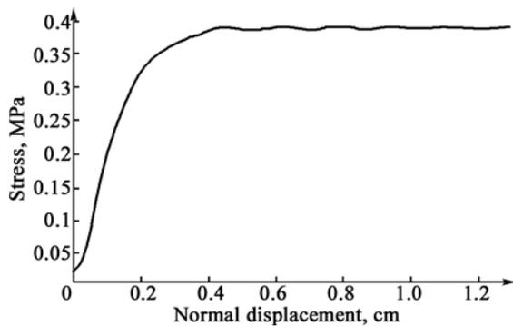
**Figure 5.** Stress–displacement relationship in the pillar without failure (when the depth of pillar is 50m and the dip of pillar is 10°)
