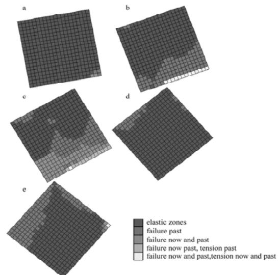
Figure 4. Failure state of coal pillar according to dip of pillar at the depth 50m
