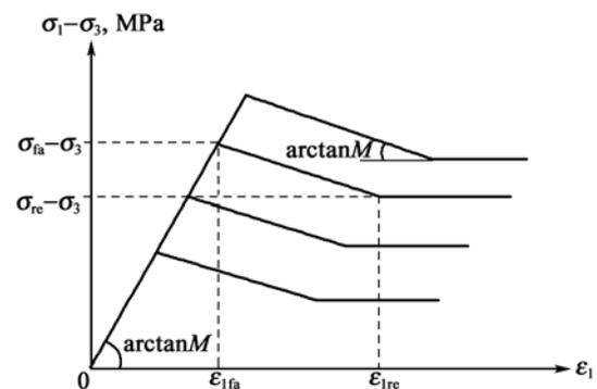
Figure 1. Elasto-plastic strain softening model of anthracite coal
