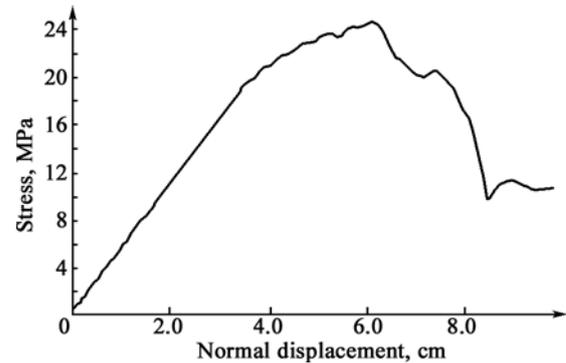
Figure 3. Complete stress-displacement curve of coal pillar at the depth of 215m
