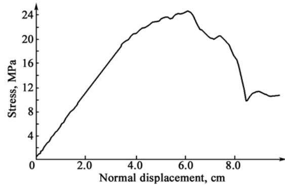
**Figure 6.** Complete stress–displacement curve of a coal pillar with the depth of 75m and the dip of 30°
