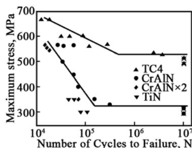
Figure 2. Fatigue test results in terms of the  $S-N$  data for the TC4 substrate and coated specimens. (Crosses mean over  $10^7$  fatigue cycles without failure).
