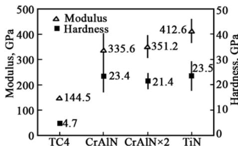
Figure 1. Elastic modulus and hardness of materials.
