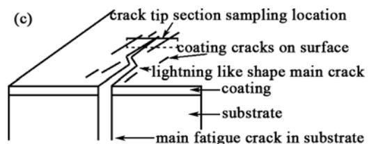
Figure 3. SEM of (a) cross section morphology crack tip and (b) non–propagating cracks in CrAlN coated sample surface, tested under 500 MPa and stopped manually when the cracks propagated to about 500  $\mu\text{m}$ ; (c) sketch map of crack tip section sampling location.
