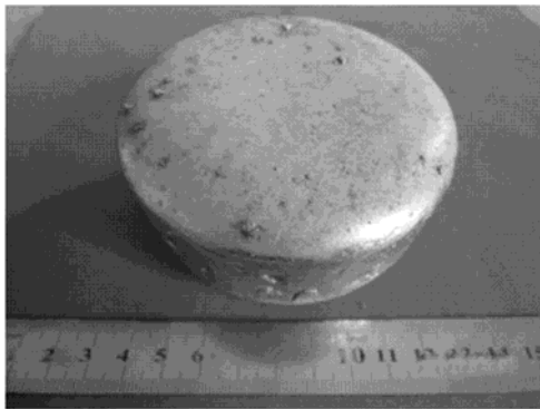
Figure 5. An alloy ingot obtained by magnetic suspension melting [19]
