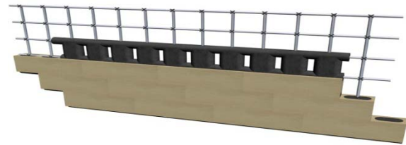
Figure 1. Double insulated cavity EPS module
