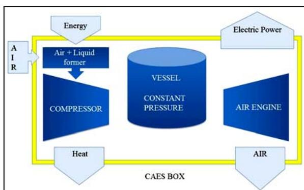
Figure 7. Scheme of a quasi-isothermal micro-CAES.
