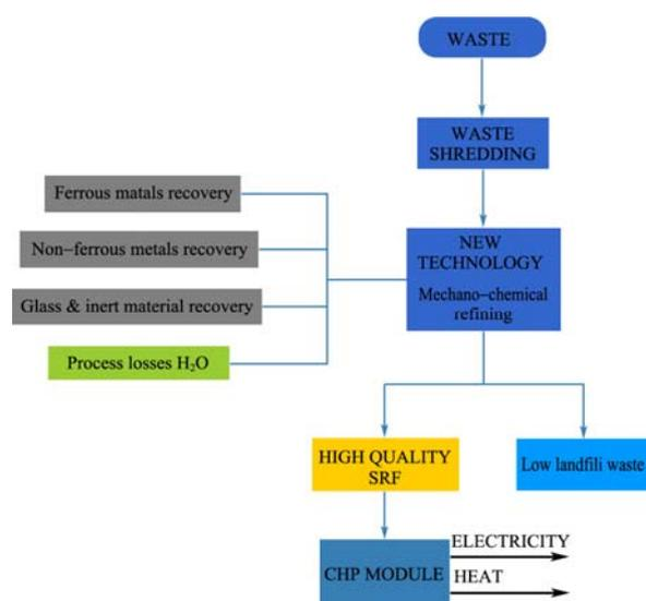
**Figure 1.** Mechano-chemical refining system.
