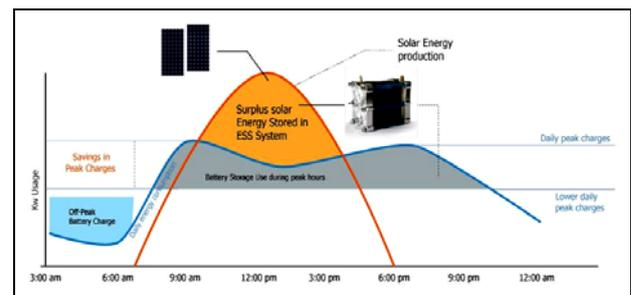
Figure 6. Peak shaving and load leveling by using RES and ESS.
