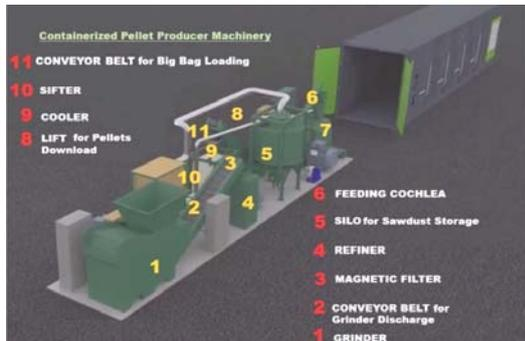
Figure 3. Design of unit 1 (waste treater – SRF production).
