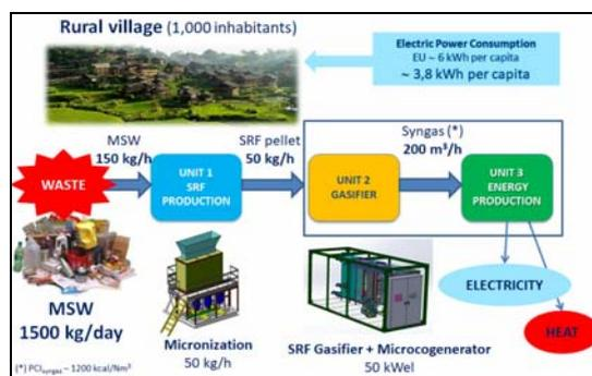
Figure 4. application of mobile platform for waste-to-energy tailored for a small rural village.
