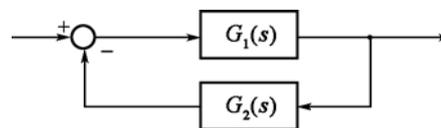
Figure 1. Block diagram of feedback system
