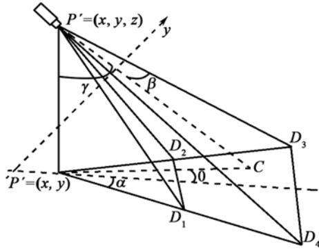
**Figure 1.** The multimedia sensor can be expressed as five elements  $(P, \bar{D}, A, \alpha, \beta)$ .
