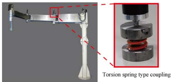
Figure 2. Overview of a partner robot and torsion spring typed coupling.
