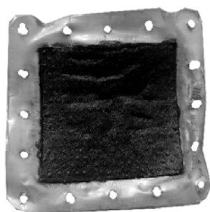
Figure 1. MEA after 1 000h(total) operation at room temperature and 0.5A/cm 2
