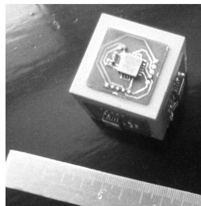
Figure 2. Sensors mounted orthogonally on three sides of a single cube (size 4×4×4cm)
