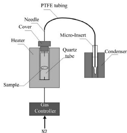
**Figure 1.** Schematic of the semiconductor condenser and heater in micro extraction Apparatus.
