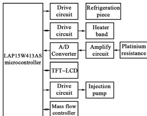
Figure 2. Electrical schematic diagram of micro extraction Apparatus
